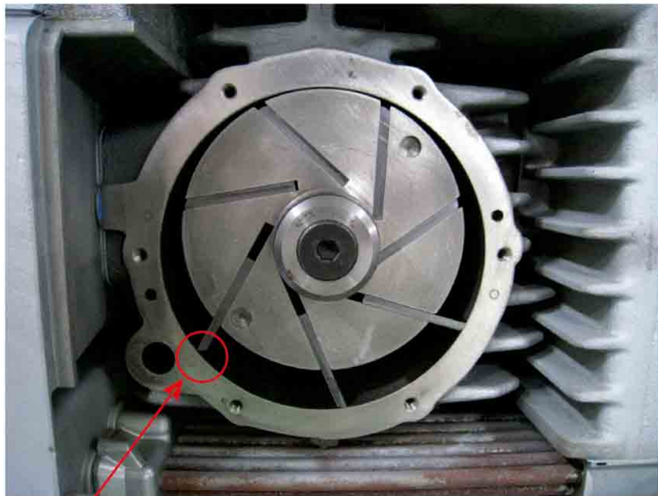
The carbon vanes are installed by incorrect direction.
